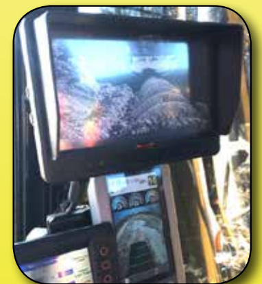
Cab monitor provides ease of viewing inside culvert
